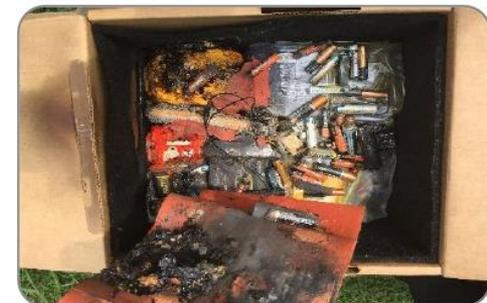
**Watch for Lithium Ion or Lithium batteries that show signs of damage such as swelling, smoking, leaking or overheating.**
